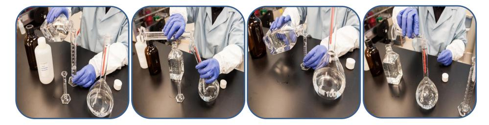
3. Add purified water to the volumetric flask and dilute to the 1,000-ml volume mark.
