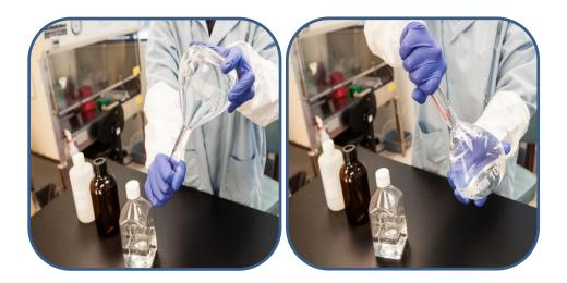
5. Transfer the diluted solution to a 1,000-ml nontransparent plastic or glass container with a tight closure (e.g., an amber-colored glass bottle or a white or opaque plastic bottle).
